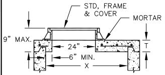
FLAT SLAB SHALL BE USED WHEN DEPTH DOES NOT PERMIT USE OF TAPER UNIT.
