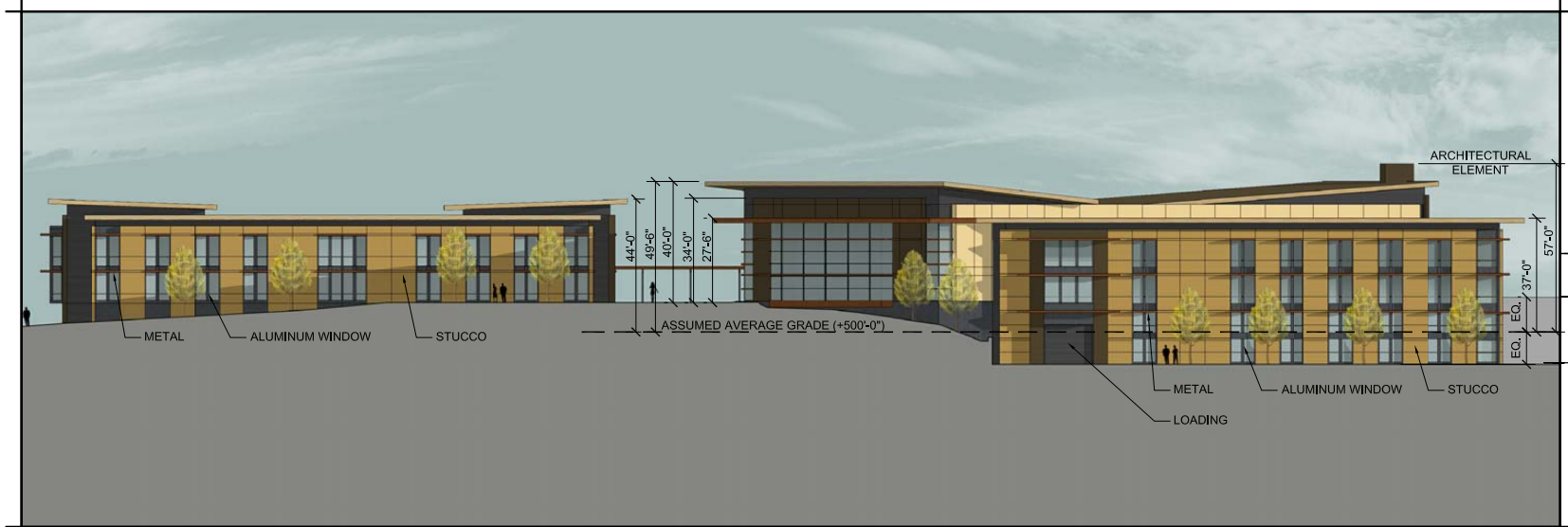
CHURCH AND ADMINISTRATION BUILDINGS: SOUTH ELEVATION
