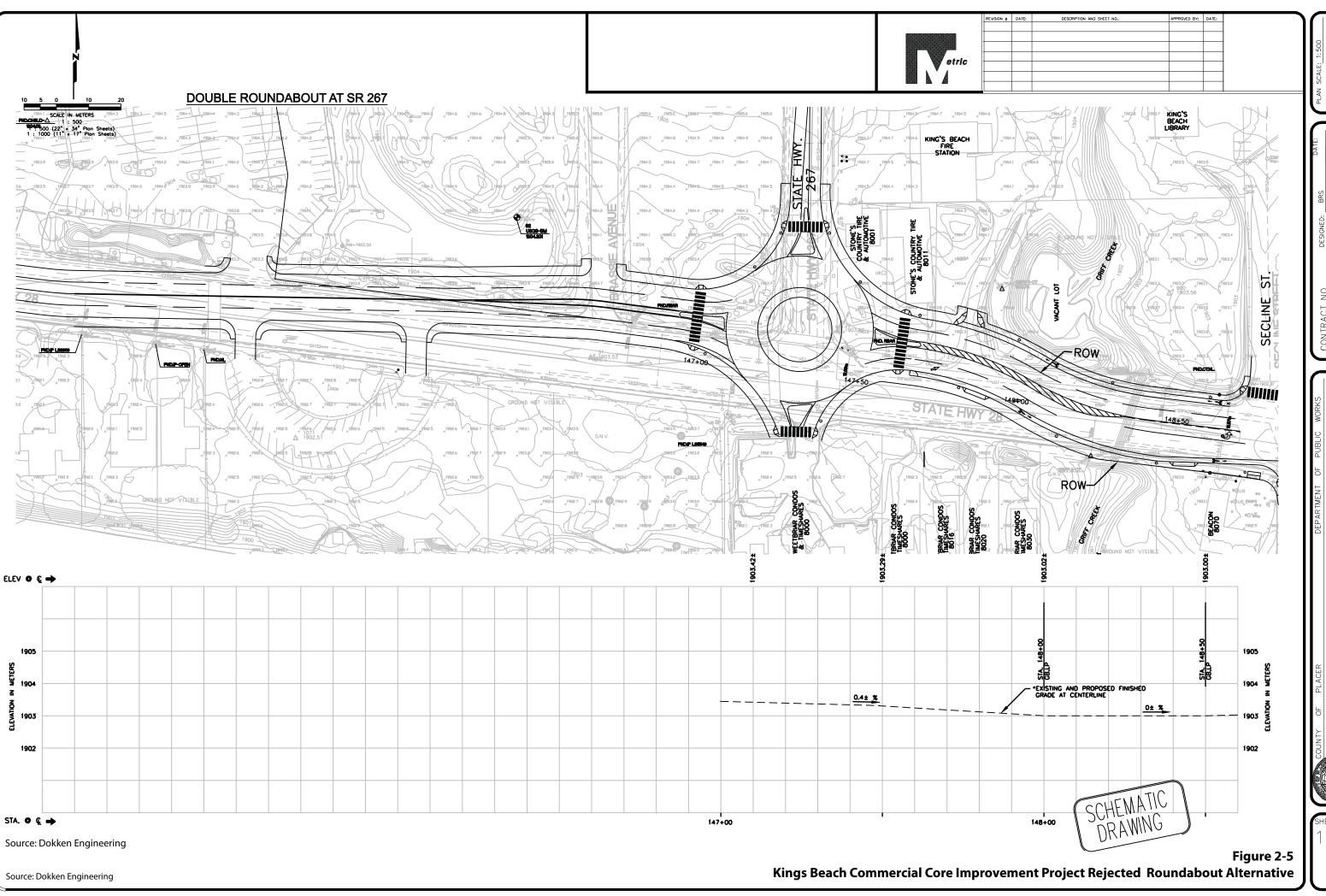
COMMERCIAL CORE IMPROVEMENT PROJECT DY - ALTERNATIVE 2 - PLAN, PROFILE & STRIPING LAYOUT
