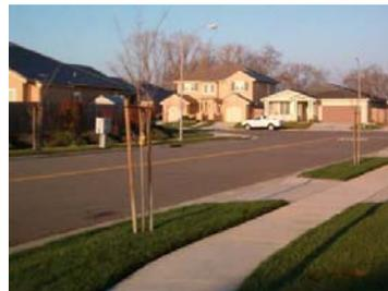
Disconnected pavement is any impervious pavement designed to sheet flow runoff over adjoining vegetated areas or porous pavement before it reaches the storm drain system.
