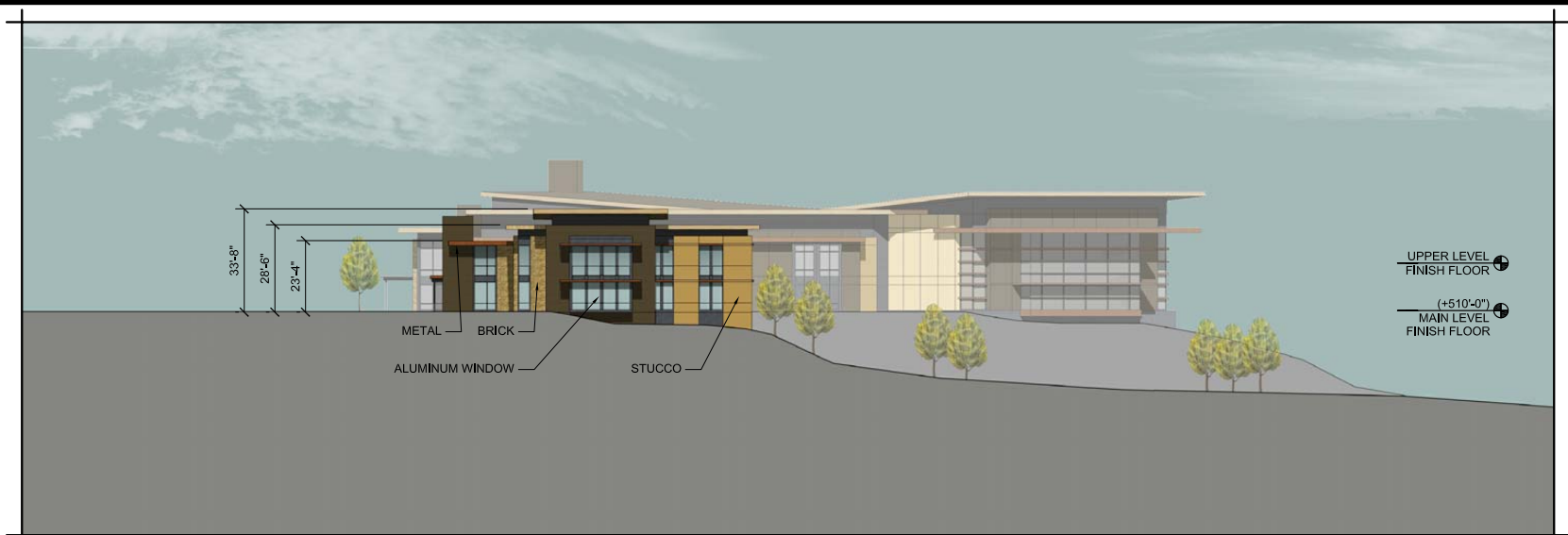
ADMINISTRATION BUILDING: WEST ELEVATION
