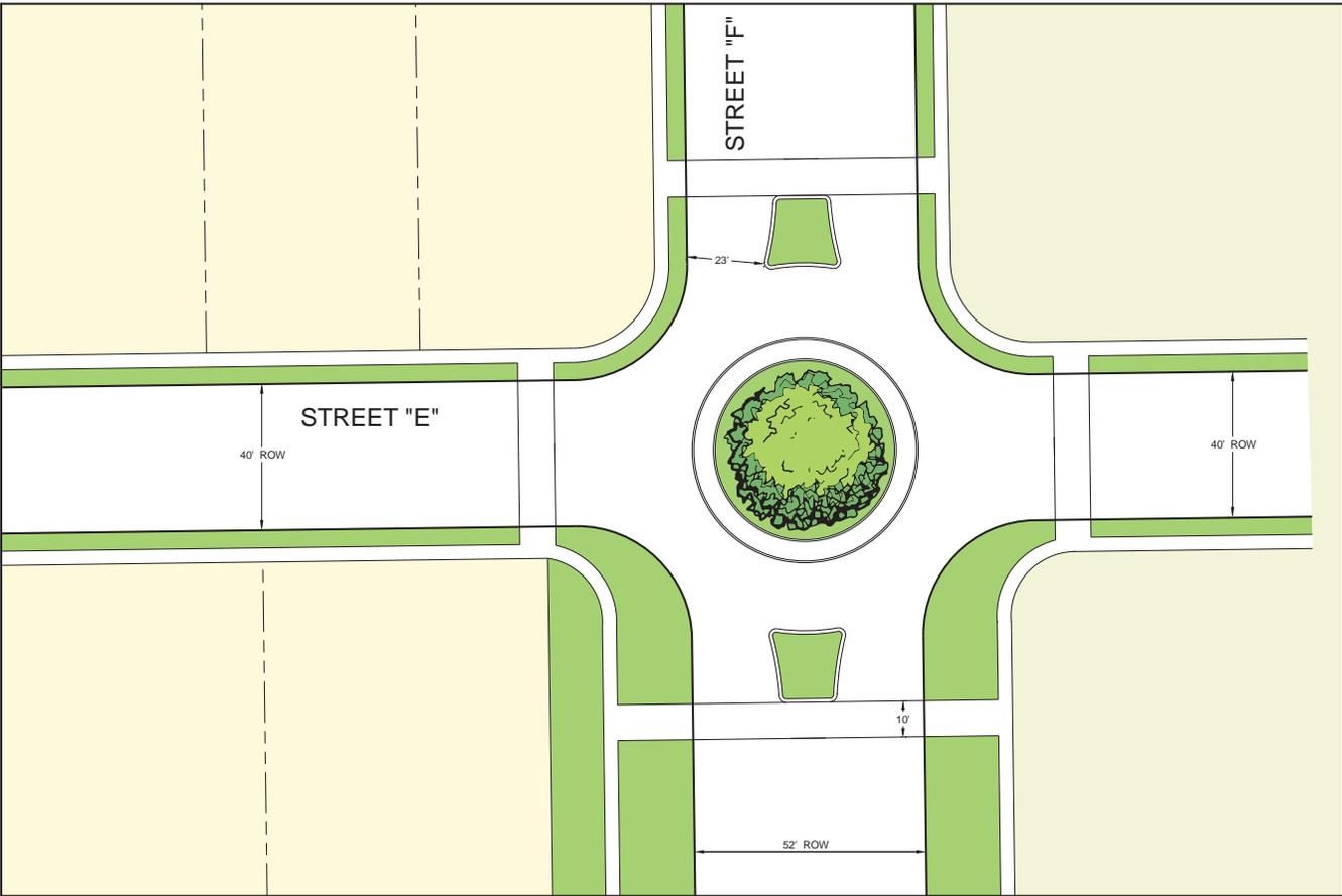
**FIGURE 4.4** CONCEPTUAL TRAFFIC CIRCLE "B" DETAIL
