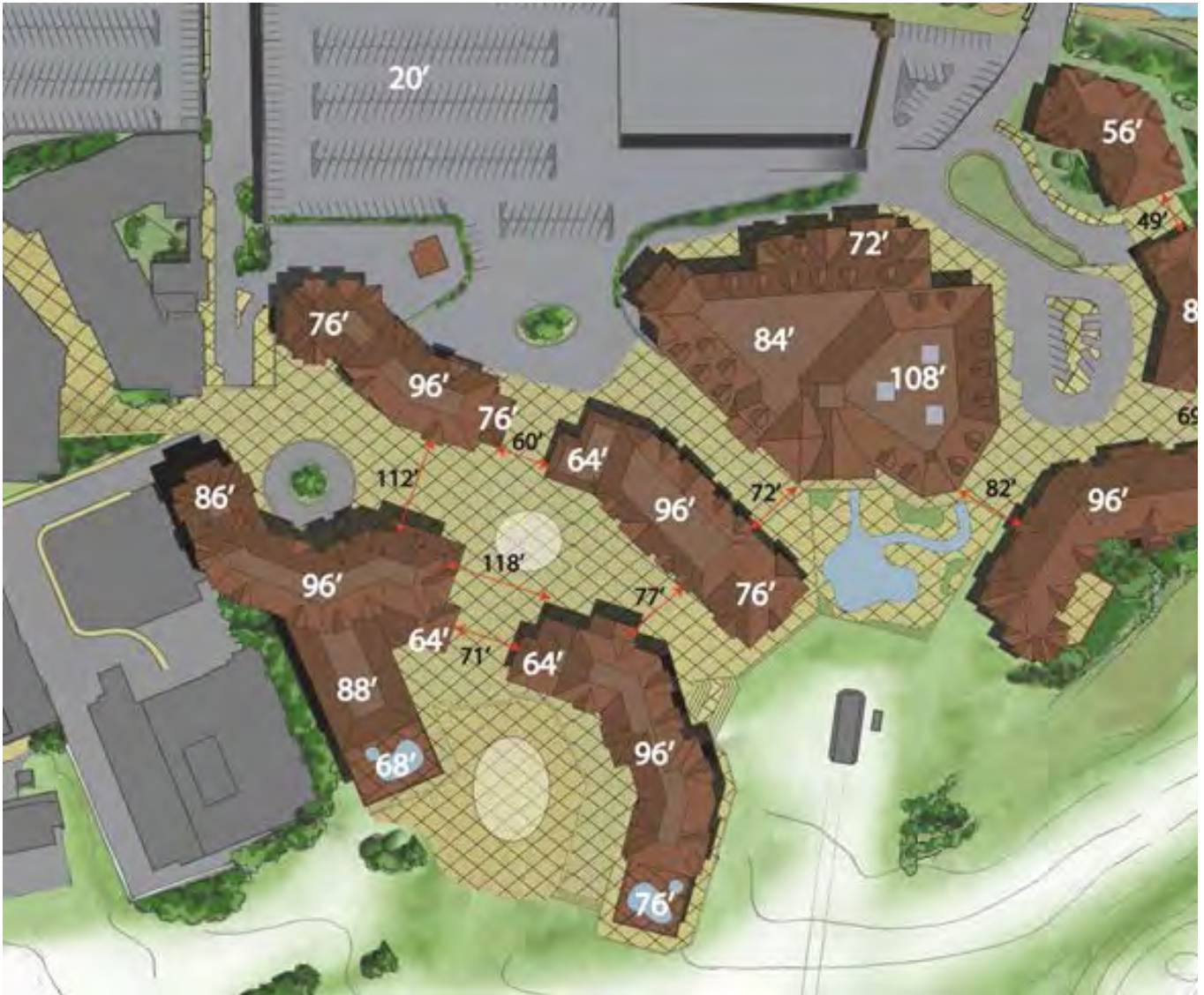
Figure 2 : Village at Squaw Valley VC-C Layout, Separations, and Heights – SVRE Response to DRC Sept 2015
